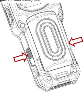
2. Pull up the bottom of the battery to remove from the device and release the battery lock
