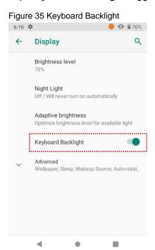
You can adjust the brightness of the keyboard backlight with the keypad. See Keypad – Functions.
