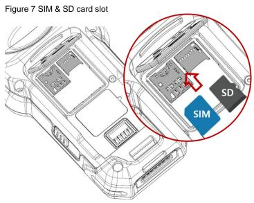
4. To remove the card, gently slide it out of the slot
