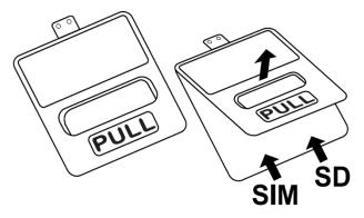
3. Referring to **Figure 7**, insert the cards in the correct orientation. Facing down the gold contact of the cards, insert a micro SIM card on the left and a microSD card on the right.
