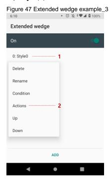
4. Tap ADD and select Move to start to point the start of the decoded data. And then, add another action of which action type is Send string and set value as "Point Mobile". Now you can get decoded data with "Point Mobile" text.
